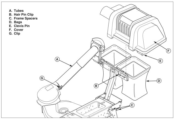
Figure 11. Normal Removal & Installation (Prestige Shown)
